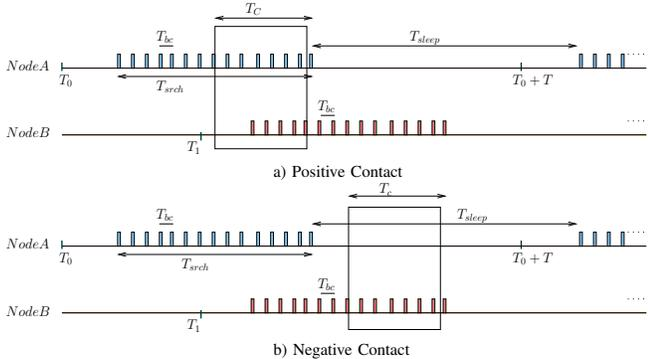
Figure 2. Contact between two nodes with Power Saving Management based on Search/Sleep duty cycling. A node switches on the wifi card at the beginning of the  $T_{srch}$  interval. A contact with other node starts at the beginning of  $T_C$  interval.
